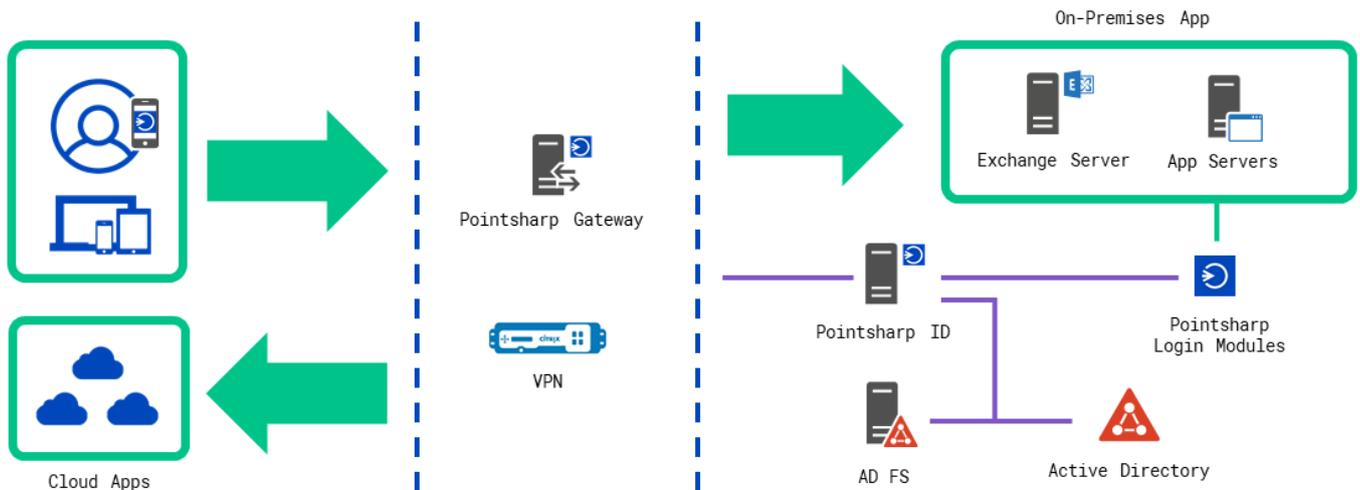
Pointsharp provide software that run on Windows Server, with the choice of deploying in your on-premises or cloud infrastructure. A non-redundant deployment exist of two instances, the internal Pointsharp ID and the Gateway placed on a DMZ. It's a split security design that meet Enterprise security requirements. Redundancy is easily achieved by multiplying the servers.
